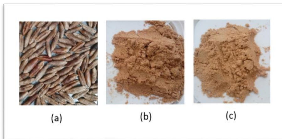
Figure II.1: Types de renfort utilisés : (a) ND (b) FND250 \mu m (c) FND180 \mu m.
