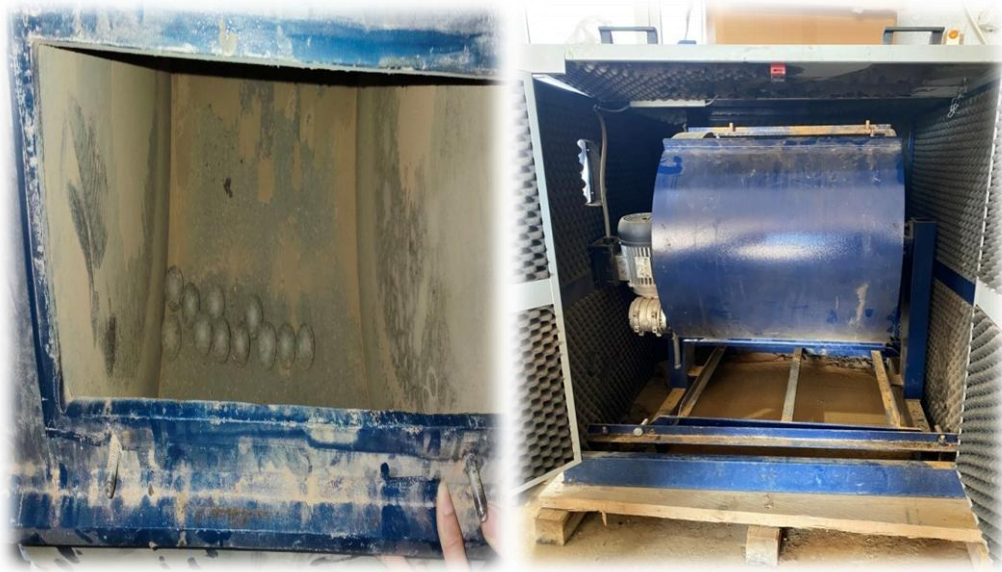
Figure II.14 : Essai los Angeles
