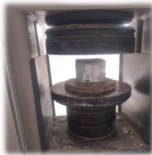
Figure II.22: Essai de compression
